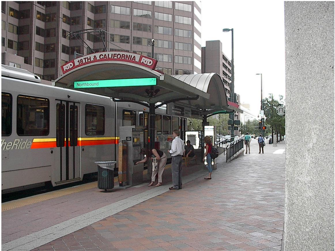
The photo above shows a typical station in downtown Denver where the platform is integrated with the sidewalk. Note that since the Denver LRVs are not true low floor cars (they have steps inside the cars) there is a need for a ramp to provide handicapped access to the head end of the train. It is intended that low floor LRVs for the SE line would be fully accessible and this type of facility would not be required. Overall the station platform amenities are very modest.
