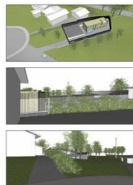
Option 3 is similar to Option 2 in that it features a recessed footprint. The site features no ramp, and as such the height of the substation relative to the street is increased. The cost is comparable to Option 2.
