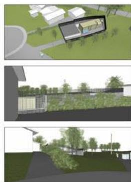
Features a recessed footprint, with retaining walls keeping the height of the substation at a minimum. It is the most expensive option.
